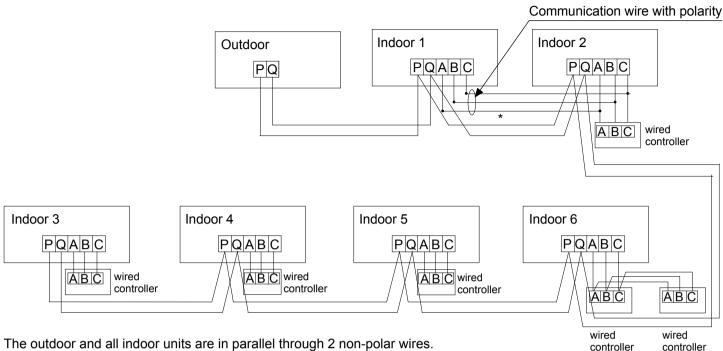
Three wiring methods between wired controller and indoor unit:
