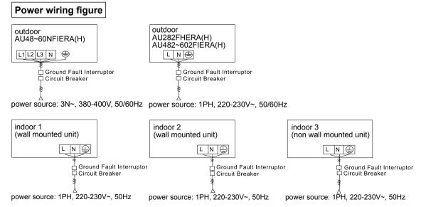
Indoor and outdoor use their individual power source. All indoors use one power source. Must install the leakage breaker and the over current breaker, or electric shock will occur.
