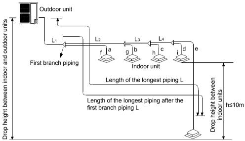
AU282 type: Maximal length and drop height permissible of refrigerant piping
