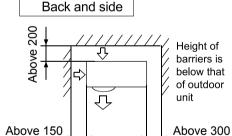
The top and two side surfaces must be exposed to open space, and barriers on at least one side of the front and back shall be lower than the outdoor unit.
