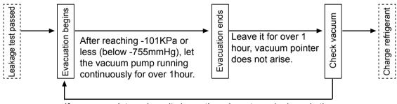
If vacuum pointer arises, it shows there is water or leakage in the system, please check and modify it, and then evacuate again.
